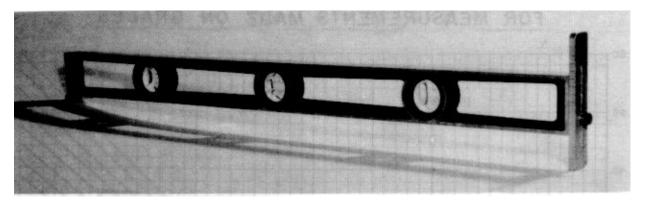
FIGURE 4 - LEVEL FOR MEASURING PAVEMENT SLOPE
