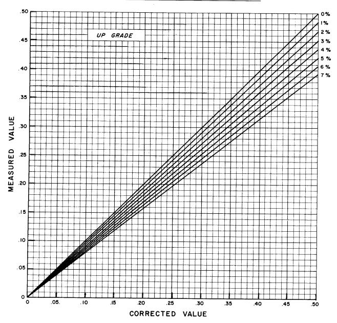
FIGURE 6 - GRADE CORRECTION CHART (UP GRADE)
