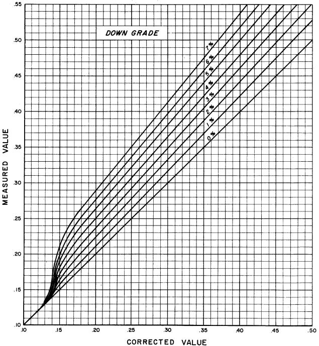
FIGURE 7 - GRADE CORRECTION CHART (DOWN GRADE)
